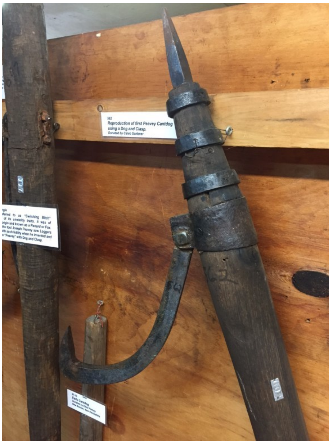
Cantdogs were essential tools for turning and handling logs in sawmills. Ian Aldrich
